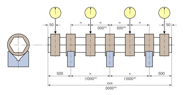
\*) Arrangement of the measurement points and of the prisms for a 3 meter bar
